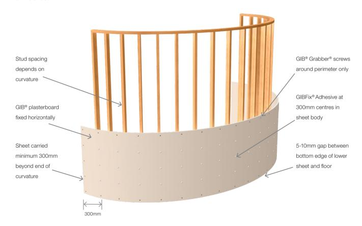
**Note** For performance systems, refer to relevant specification sheet for the fastener and nog requirements.
