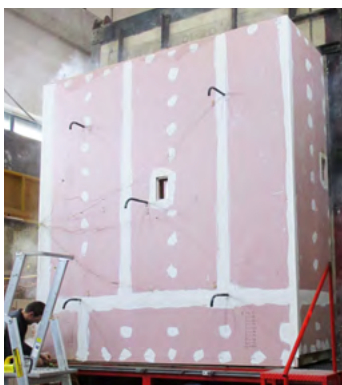
(a) Extended furnace beyond the specimen
