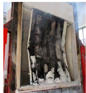
(c) Residual timber-framed wall
