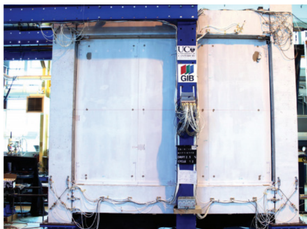
FIGURE 2: Non-structural partition being tested at Canterbury University
