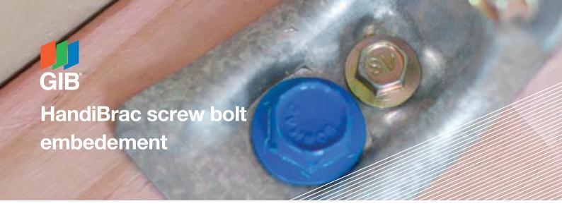
GIB® bracing elements requiring special hold-down fixings at panel ends are identified with an 'H', i.e. GSP-H, BL1-H, BLG-H and BLP-H. When load is applied to the top of high-performance elements, the end study need to be anchored to stop the panel from 'tipping'.
