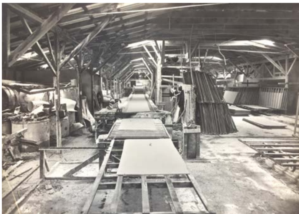
TOP LEFT: 1930 th – There are big improvements – the wallboard is now cut at its required length before going to the drier. The edges are already sealed so that no further trimming is needed. BELOW: Early wallboard production process.
