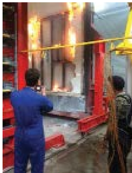
LEFT: Steel studs glow red-hot immediately following a pilot-scale furnace test. MIDDLE: A timber framed specimen at the end of a full-scale furnace test. RIGHT: Thermocouples collect important temperature data.
