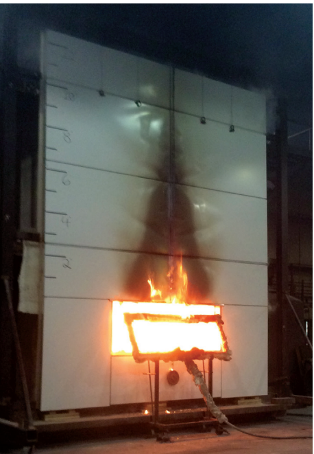
ABOVE LEFT: Fire test in progress. ABOVE MIDDLE: Completed fire test with cladding still in place. ABOVE RIGHT: Completed fire test with cladding removed and GIB Weatherline® visible.
