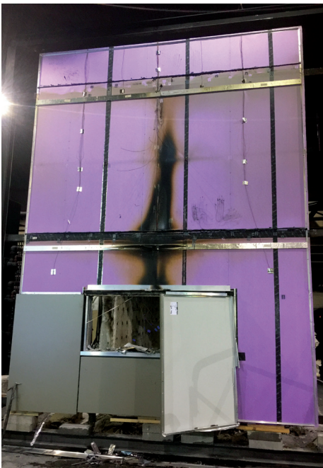
ABOVE LEFT: Fire test in progress. ABOVE MIDDLE: Completed fire test with cladding still in place. ABOVE RIGHT: Completed fire test with cladding removed and GIB Weatherline® visible.
