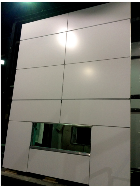
ABOVE: Preparation for the fire test with GIB Weatherline® lining (left) and with cladding (right).
