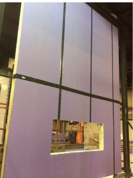
ABOVE: Preparation for the fire test with GIB Weatherline® lining (left) and with cladding (right).
