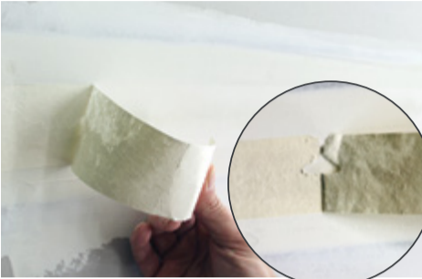
FIGURE 5: Inadequate compound under the tape and the tape can be removed relatively clean and easily.
