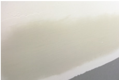
FIGURE 1: Basecoat compound has a darker colour and indicates it has set properly.
