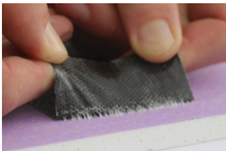
These photos show how strength builds up over the course of contact time. LEFT: 2 mins after GIB Weatherline® Flashing Tape installation. RIGHT: 20 min after GIB Weatherline® Flashing Tape installation, significantly stronger adhesive bond.
