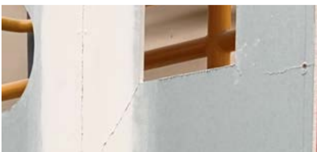
Figure 3: A close up of cracks after racking.
