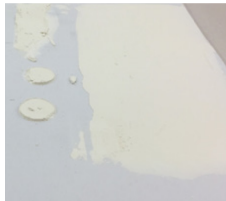
FIGURE 1: Setting compound strong joint adhesion through gypsum crystal formation.
