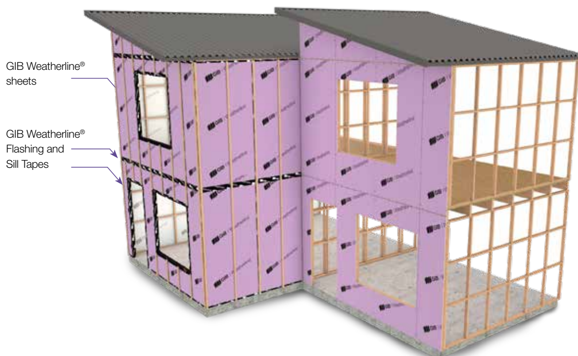
FIGURE 1: TYPICAL INSTALLATION OF GIB WEATHERLINE® SYSTEM
