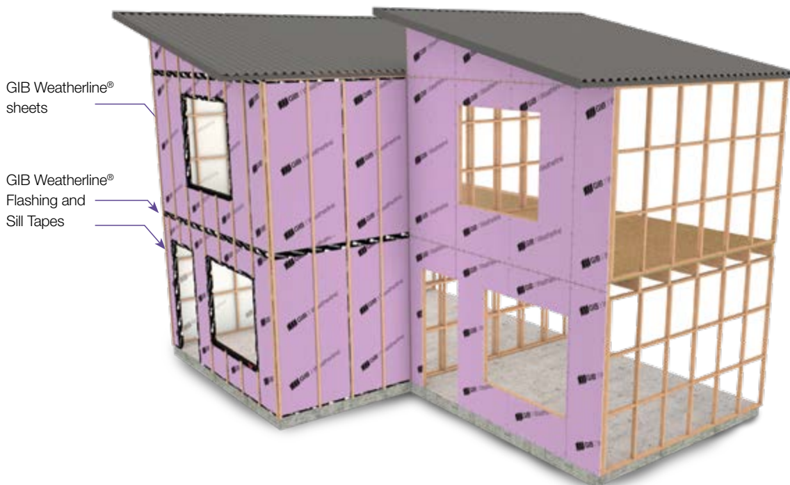
FIGURE 1: TYPICAL INSTALLATION OF GIB WEATHERLINE® SYSTEM
