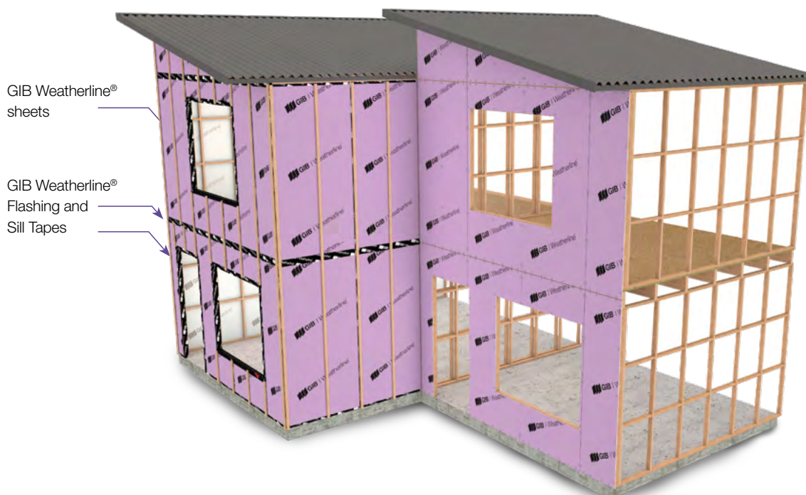
FIGURE 1: TYPICAL INSTALLATION OF GIB WEATHERLINE® SYSTEM
