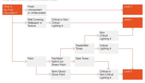
May not be suitable for subsequent decoration to high levels of quality in the future. Refer to Level 4 or 5 for upgrading requirements. # Critical lighting – when the light source is nearly parallel to the surface.
