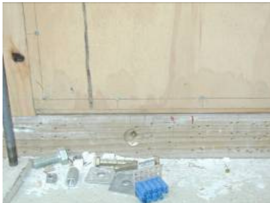
Plate 2 Bottom of Plywood Bracing Element After Testing
