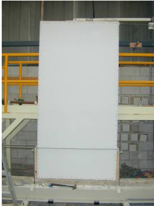
Plate 9 Refastened Bracing Element after Testing
