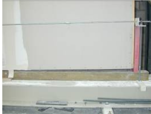
(b) Element Uplift During Testing
