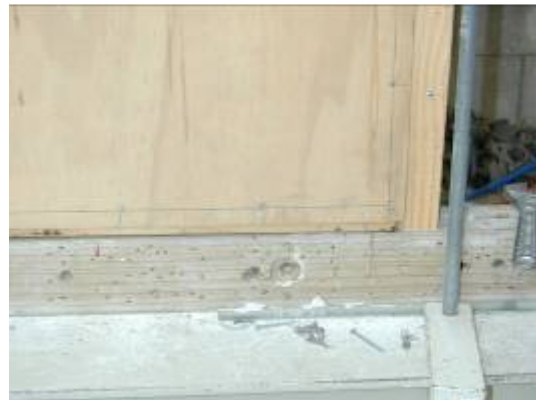
Plate 2 Bottom of Plywood Bracing Element After Testing
