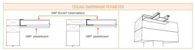
Perimeter channel, (340, 142 or 140) to be fixed with 32mm x 8g GIB® Grabber® wafer head screws at 300mm centres
