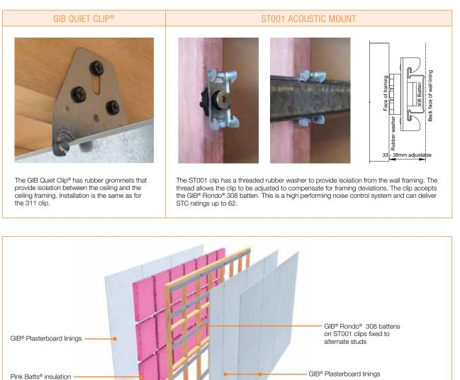
Typical usage of ST001 clip with GIB® Rondo® 308 batten in a GIB® Noise control system. For full installation details for noise control systems please refer to the publication GIB® Noise Control Systems (www.gib.co.nz)
