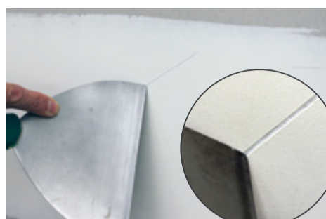
FIGURE 3: A scratch in a properly set basecoat is only super-visual and indicates it is hard.
