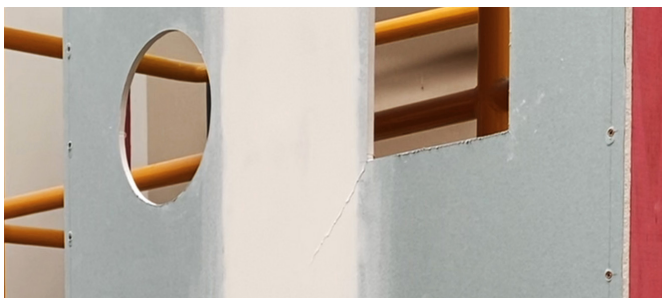
Figure 2: Test specimen during racking.
